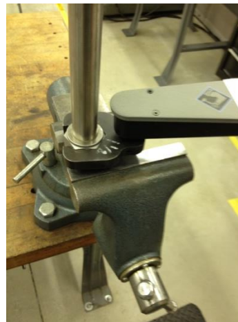
Figure 2.1.2 Initial Make-up Torque Test Equipment
