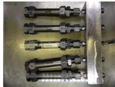
Figure 2.2.2 Gas Leak Test Configuration
