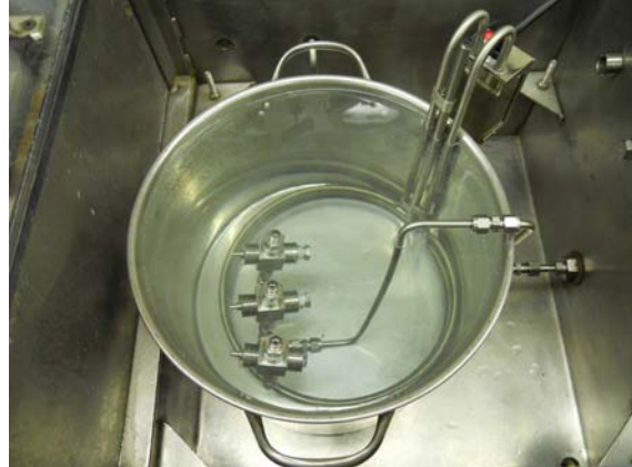
Figure 2.4.2 Leak Test set up for High Temp Test
