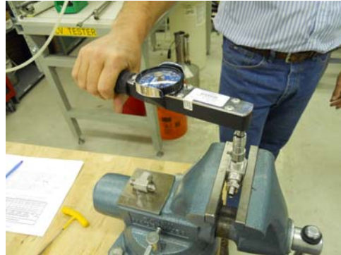
Figure 2.6.1 Torque Test Setup
