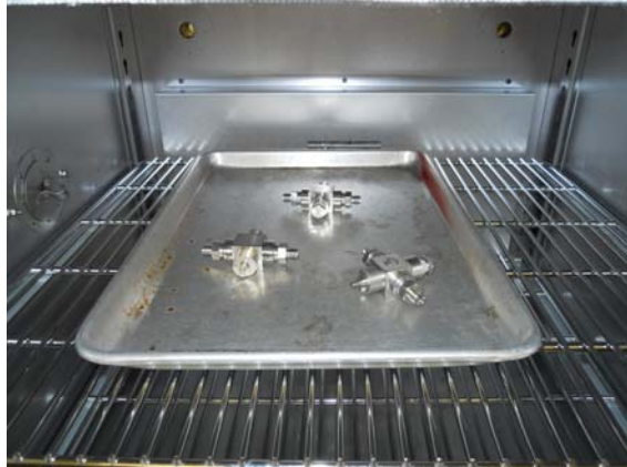
Figure 2.4.1 Leak Test set up for High Temp Test
