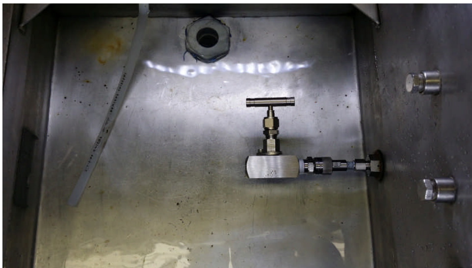
Figure 2.2 Leakage Test (Ambient) Setup
