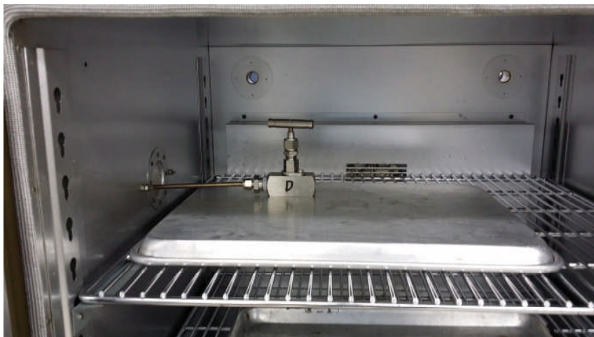
Figure 2.4.1 Leakage Test High Temperature Setup (250°F - 450°F)
