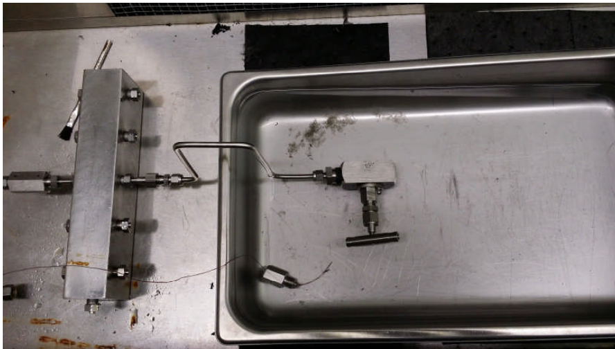
Figure 2.3 Leakage Test (Low Temperature) Setup
