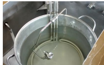
Figure 2.4.2 Leakage Test (200°F) Setup
