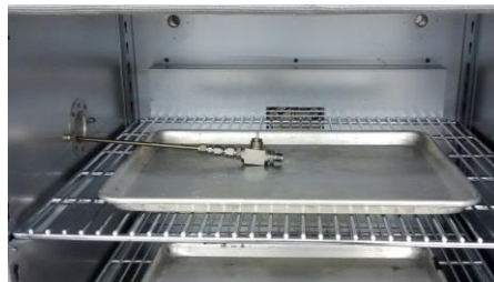
Figure 2.4.3 Leakage Test (Over 200°F) Setup
