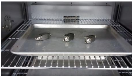
Figure 2.4.1 Leakage Test High Temperature Soak Setup
