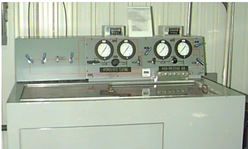
Figure 2.2.1 Gas Leak Test Equipment
