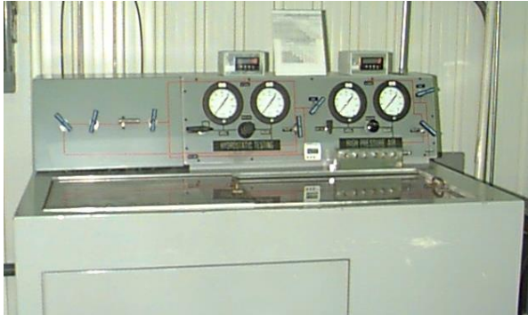
Figure 2.3.1 Burst Test Equipment
